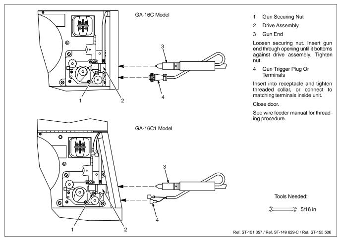
Figure 3-1. Installing Gun
